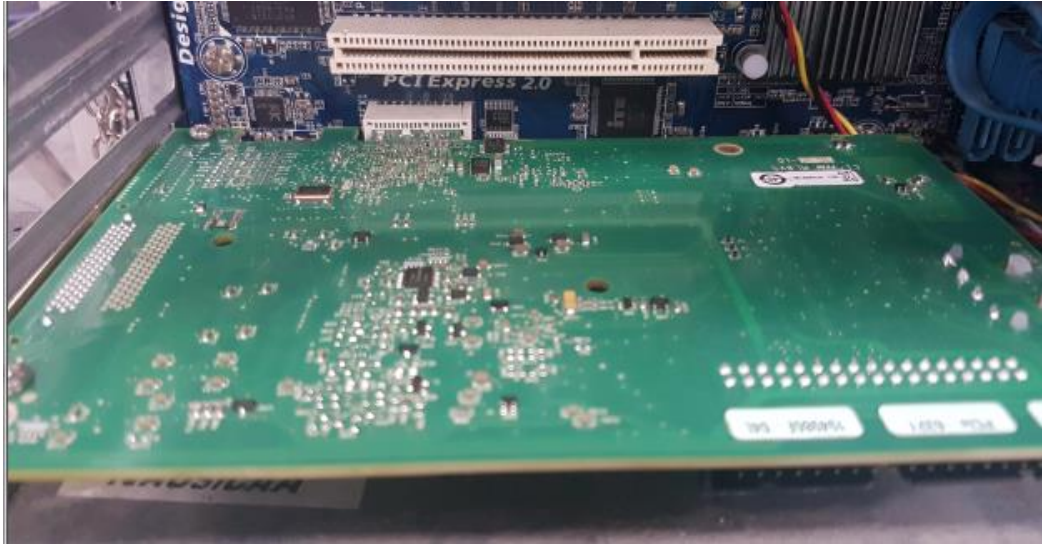
Figure 83: PIC-EXPRESS card connection
