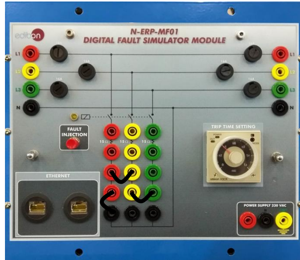
Figure 64: N-ERP-MF01 three pole to ground setting fault
