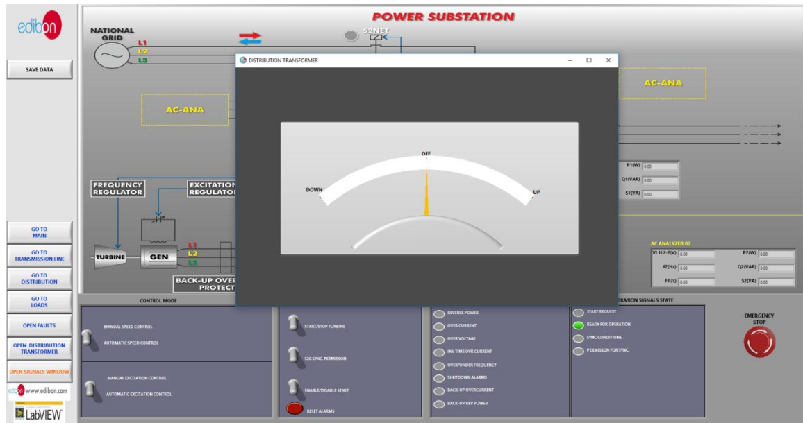
Figure 116: Voltage regulator screen for the regulating transformer control
