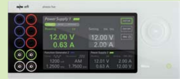
Control center + 3 regulating power supply units + functional generator
