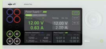
Control center + 2 regulating power supply units + functional generator
