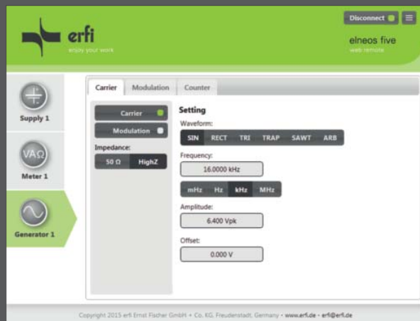
Telecontrol function generator and quick signal arbitrary generator: All parameters of the function and signal arbitrary generators are telecontrollable.
