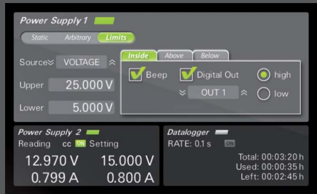
Limiters: The limiter allows the free control of all voltage and current areas in connection with limited. Each state can be coupled with an audible signal and a freely selectable digital output.
