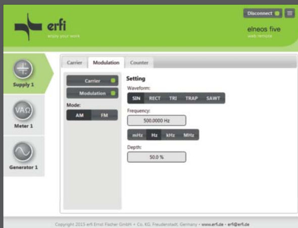
Modulation by web server: The web server allows also the telecontrol of AM, FM and PWM modulation.
