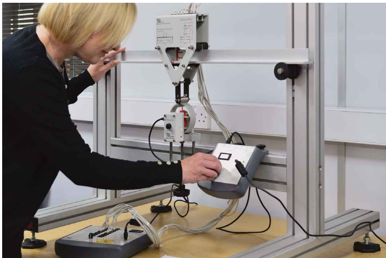
Test Frame (STR1) fitted with the experiment module Bending Stress in a Beam (STR5) and Digital Force Display (STR1a)
