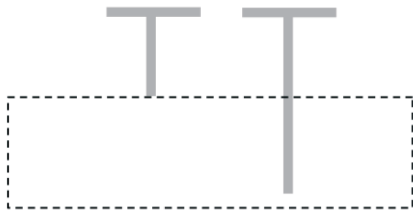
Figure 21: Brushing over the light gray lines with conductive varnish
