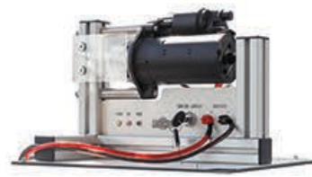
Automotive 12V Starter functional model
