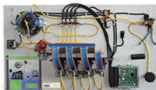
LPG TIMED SEQUENTIAL INJECTION FOR ELECTRONIC INJECTION ENGINES (wall-mounted) – cutaway training model
