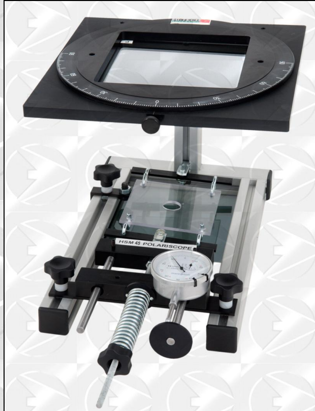
Figure 1: With Square Plate Specimen Fitted
