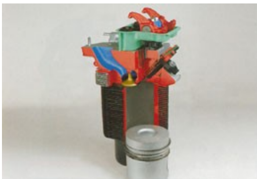
Order No. 1167 MAN direct injection with bowl-in piston
