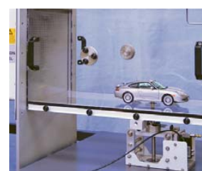
Base mounted with model car to measure drag
