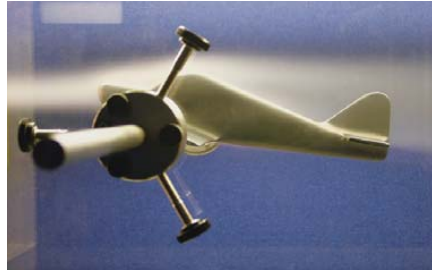
Smoke trail around the Low Wing Aircraft Model (AF107)
