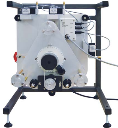
Three-Component Balance shown with the Angle Feedback Unit (AFA4)
