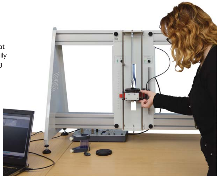
Shown fitted to the Test Frame (TM160) and connected to VDAS® mkII
