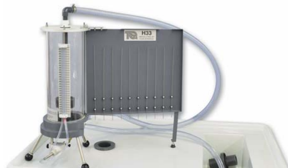
THE DIGITAL HYDRAULIC BENCH SHOWN WITH THE JET TRAJECTORY AND ORIFICE FLOW (H33) EXPERIMENT MODULE
