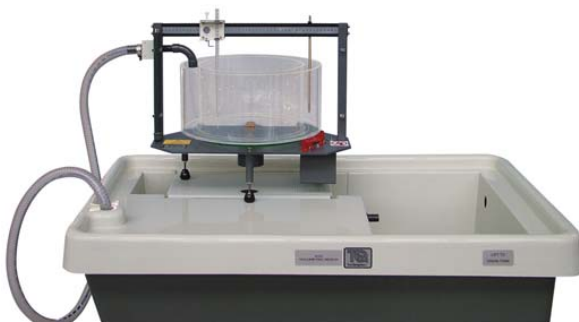
The Volumetric Hydraulic Bench shown with the Vortex Apparatus (H13) experiment module
