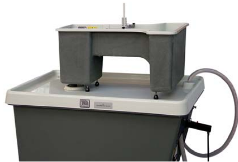
The Gravimetric Hydraulic Bench shown with the Discharge Over a Notch (H6) experiment module
